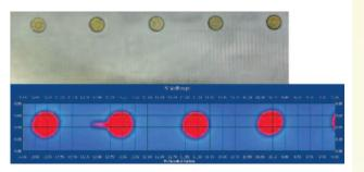
Subsurface flaw from steel fastener
