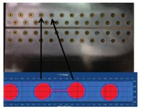
Flaw between steel fasteners
