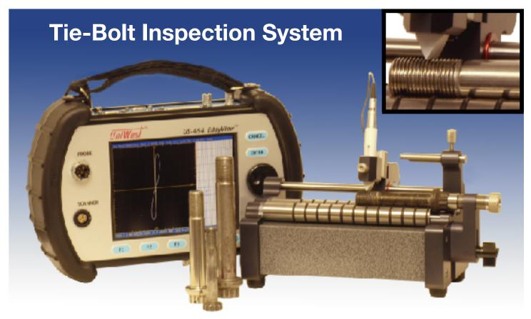
The strength of UniWest's tie-bolt inspection system is in the simplicity of the design. Using both gravity and thread angle, the probe is driven along the thread pattern and then manually manipulated along the rest of the shank and head radius. The entire inspection can be completed in less than seven seconds. There are no expensive fixtures to replace. All standard size tie bolts can be inspected with this one instrument. Special modifications can be made to fit over and undersized bolts.
